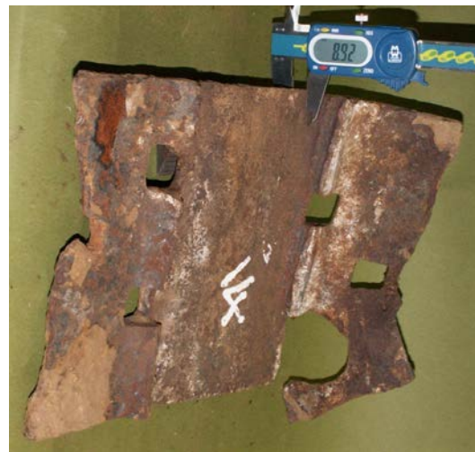
Figure 11: Typical base plate
