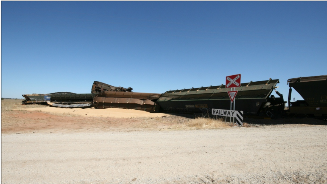
Figure 3: Derailed wagons beyond the level crossing
