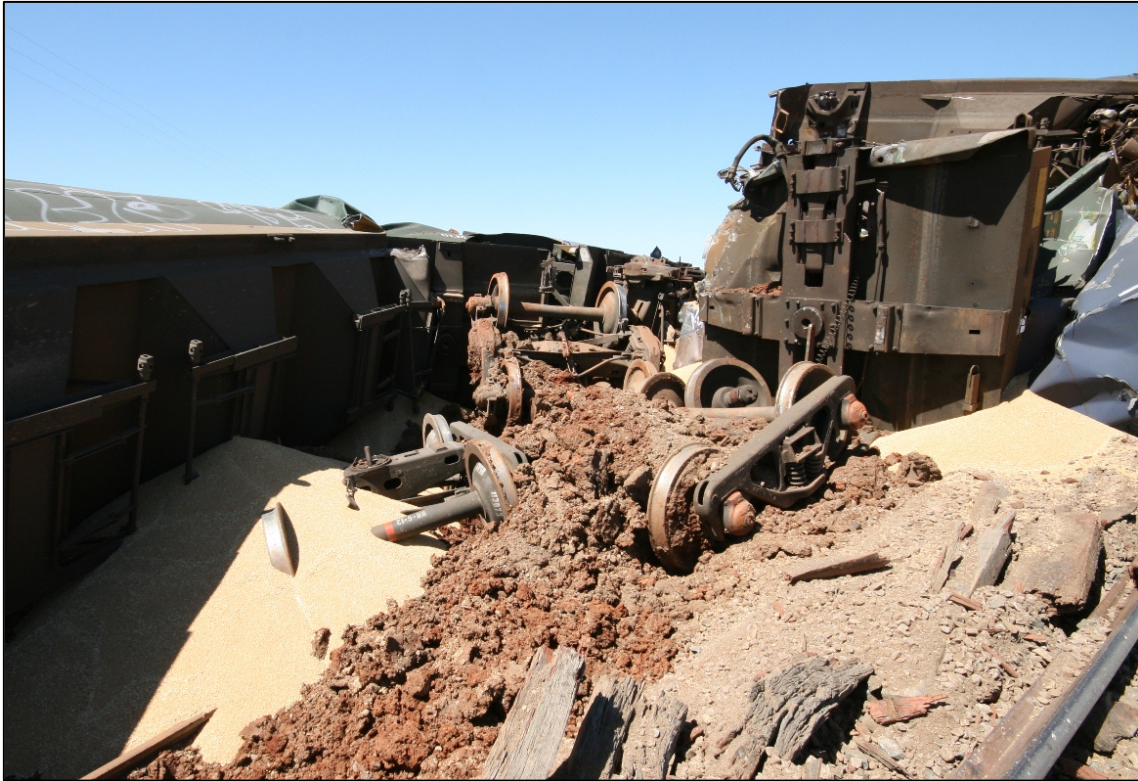
Figure 8: Extensive damage to derailed wagons
