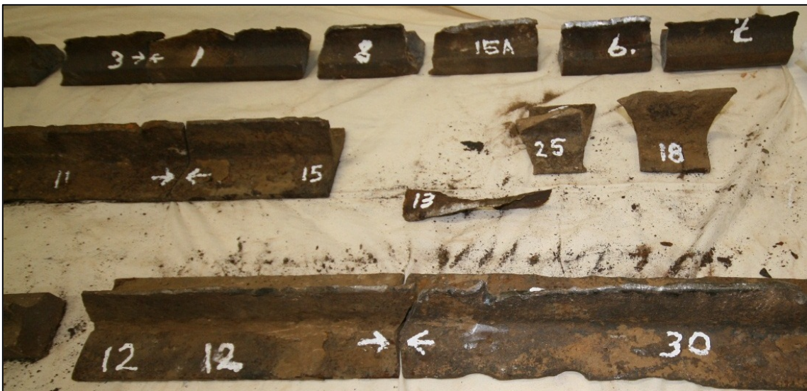
Figure 9: A selection of the fractured rail examined
