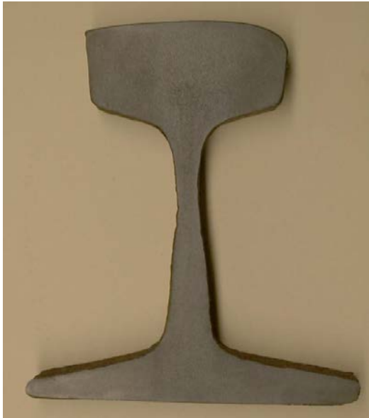
Figure 10: Wasted rail, intact section
